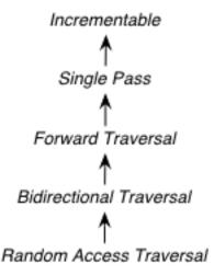
In addition to the iterator movement operators, such as operator++, the traversal concepts also include requirements on position comparison such as operator== and operator<. The reason for the fine grain slicing of the concepts into the Incrementable and Single Pass is to provide concepts that are exact matches with the original input and output iterator requirements.
